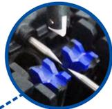
Ultra narrow ceramic V-groove, suitable for any application.
